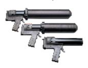
The Semco® Model 550 sealant gun is designed for the pneumatic application of sealant, caulking, adhesive, and other compounds packaged in Semco® 1/10th gallon, 20, and 32 oz.cartridges. Parts are available to convert the gun from one size to another. Air hoses to operate the gun must be ordered separately (see page 15 for more information). These lightweight guns are constructed of cast aluminum and other durable materials.
