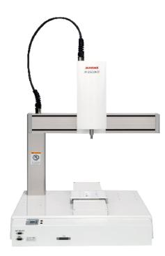
BENEFITSVersion 3 or 4 axes. Stepper motor with encoderIntegrated control systems and meteringSolid structure to ensure accuracyInterface production lineEmergency stop and resetChoose from 10 different display languagesSwitch between the coordinate values displayedExtended Memory Up to 255 programs and 30 000 pointsPossibility of an established system or standalone
