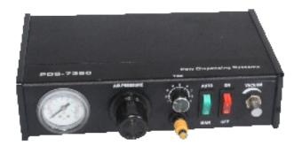
The calibrated time / pressure 7350 dispenser exists in version 0-1 bar, for highly liquid products, and 0-7 bar for other products. It is equipped by a MAC solenoid valve offering a constant flow rate and adjusting dispense time in hundredts of seconds.
