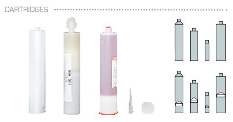
Disposable plastic cartridges are available in 1, 2.5, 6, 8, 12, 20, 32 oz. (approximate metric value 30, 65, 170, 230, 340, 610, 950 cc ) and 1/10th gallon capacities. Available in low or high - density natural polyethylene, all sizes are fit with 1/4» NPT (6mm) female thread dispensing orifice. Special colours are available, however minimum order, lead time, and pricing considerations apply.
